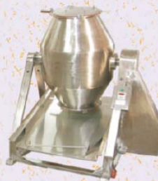
Mixer Machine : Ues For Tea, Namkin, Washing Powder, Spices, Granul Etc. Capacity - 50, 100, 250 And 500 Kg.
