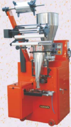
Central And Three Side Pouch Packing Machine, Cap. 1gr. To 1kg.
