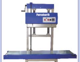
Continue Bag Sealing Machine (Heavy Model) Up to 15Kg.
