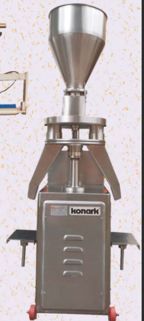
Filling Machine Two Head Cap.50 to 500 gr.
