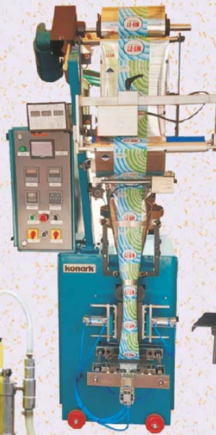
Pneumatic Pouch Packing machine Cap.10 to 500 gr.
