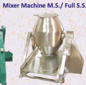
Mixer Machine : Ues For Tea, Namkin, Washing Powder, Spices, Granul Etc. Capacity - 50, 100, 250 And 500 Kg.
