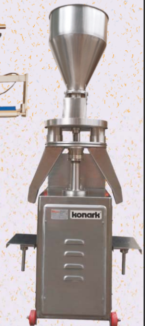
Filling Machine Two Head Cap.50 to 500 gr.
